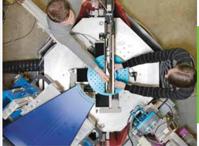
Neutron investigation of turbine blades: owing to research cooperation with PSI, Alstom will in future be able to avoid material fatigue in high-performance turbine blades. (Photo: Scanderbeg Sauer Photography)
