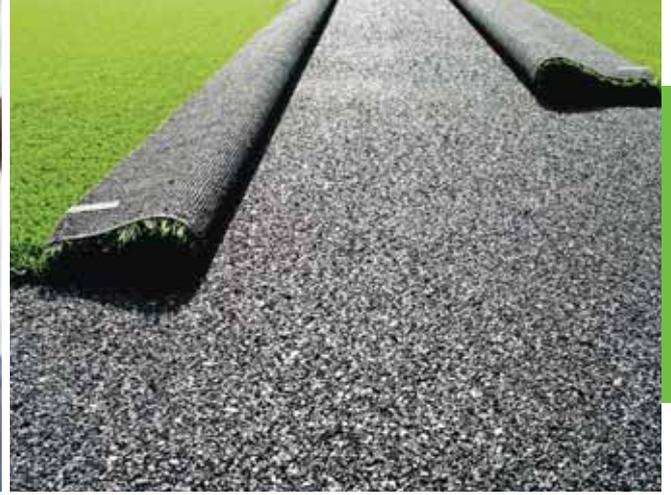
Ongoing accreditation process at FIFA: the floor manufacturer Tisca Tiara and Empa jointly developed an artificial turf whose "blades of grass" stand up again and have a low sliding friction.
