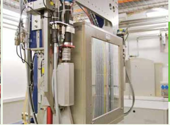
Highly sensitive x-ray detectors for synchrotron applications: after successful tests, Dectris and PSI are jointly developing a marketable next detector generation within the scope of a CTI project.
