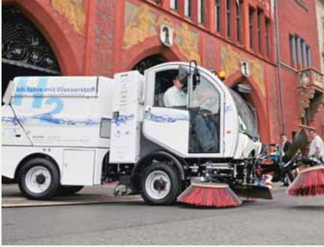
Energy-efficient propulsion technologies: after the successful hydrogen propulsion system for communal vehicles, Bucher Schörfling and Empa jointly developed a hybrid propulsion system within the scope of a CTI project.
