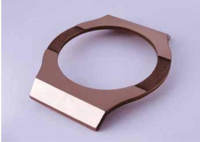
Unscratchable gold: in cooperation with the watch-making company Hublot, researchers at EPFL have developed gold that is harder than steel. This 18-carat gold is an alloy with boron carbide (Photo: Hublot)
