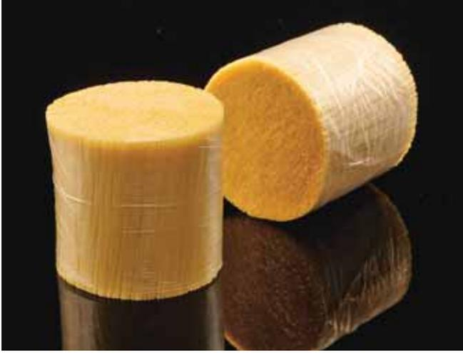
Favourably priced, simple concrete reinforcement: Brugg Seiltechnik Holding AG and Empa developed bi-component fibres from polymers, which can be mixed into concrete to provide it with a high load capacity. (Photo: Brugg Contec AG)
